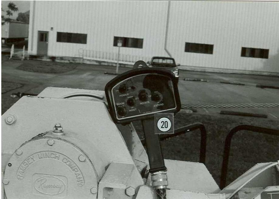
20. Crane Hand Controls- A remote hand control unit used to control all crane functions. When plugged into the left rear side of the crane, the operator has the ability to control the Boom up/down, Hoist up/down, Rotation cw / ccw, or Boom Extend in/out. There is also a Power on/off switch which when left unattended should remain in the “off” position.
