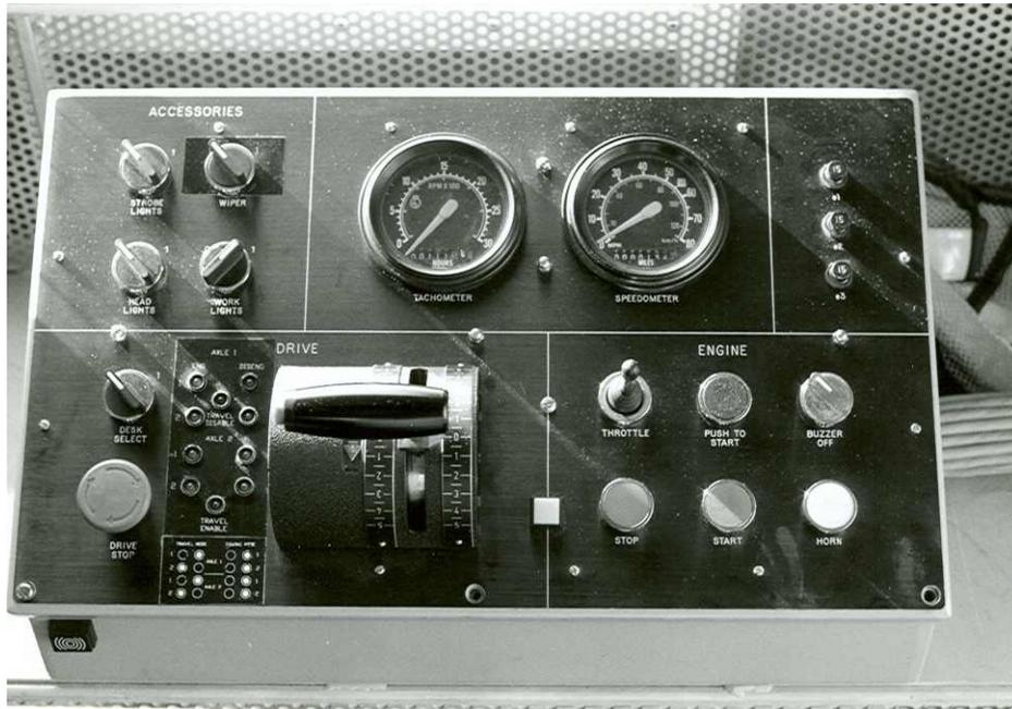
The B11 auxiliary drive control panel has the same controls on it as the B5 panel. This driving desk is at the rear of the cab and is used to travel the machine in a rearward direction.
